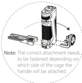
Note: The correct attachment needs to be fastened depending on which side of the cage the handle will be attached.
